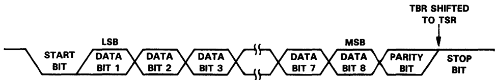
Figure 3-32. Asynchronous Transmission of Eight Bits Plus Parity
